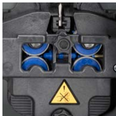
4-roll wire-feed system (Automig 273)
