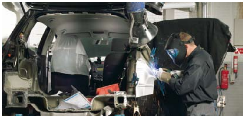
MIG/MAG welding in sheet metal
