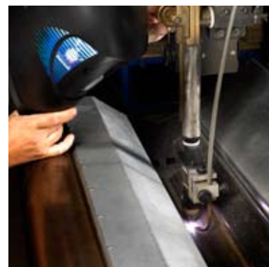
Plasma welding of stainless material in a long-seam automated device
