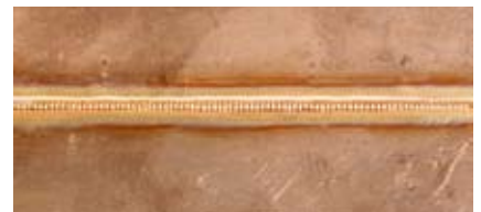
Copper – plasma-melt in 0.6 mm wall thickness
