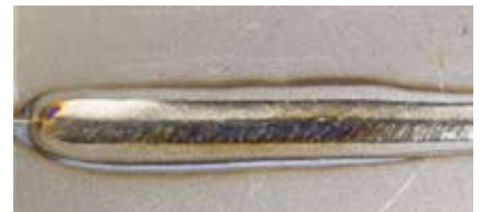
Stainless steel – Plasma-keyhole welding in 6 mm wall thickness
