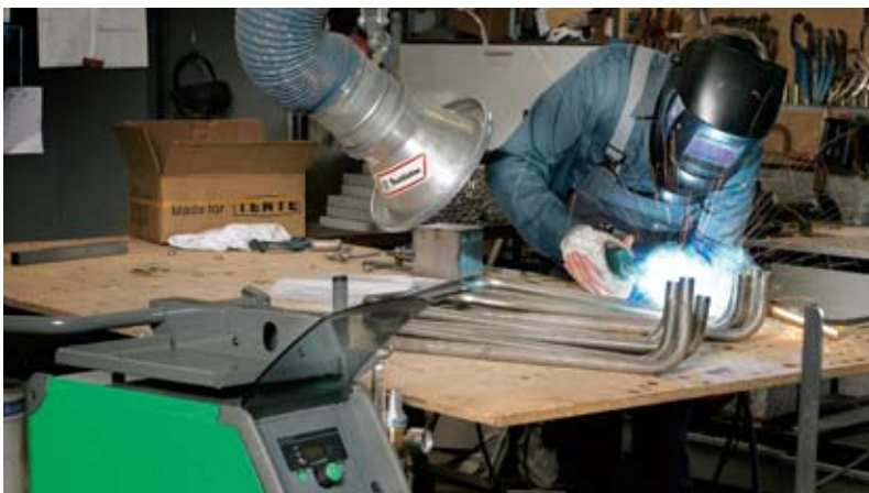
Construction of food industry equipment, using DUO Plus in stainless material
