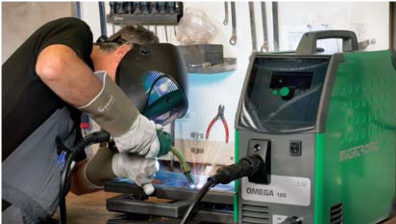
Welding of profiles for furniture frames in mild steel
