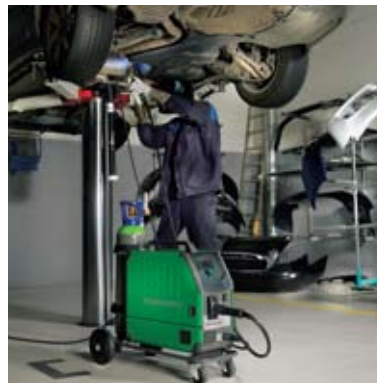
Repair of exhaust pipe suspension
