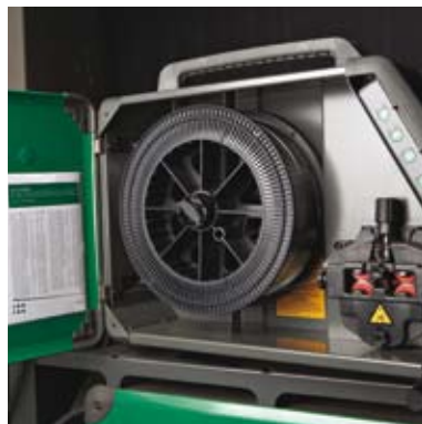
Wire feed unit with four-spool wire feeding and colour-coding - simple and logical.
